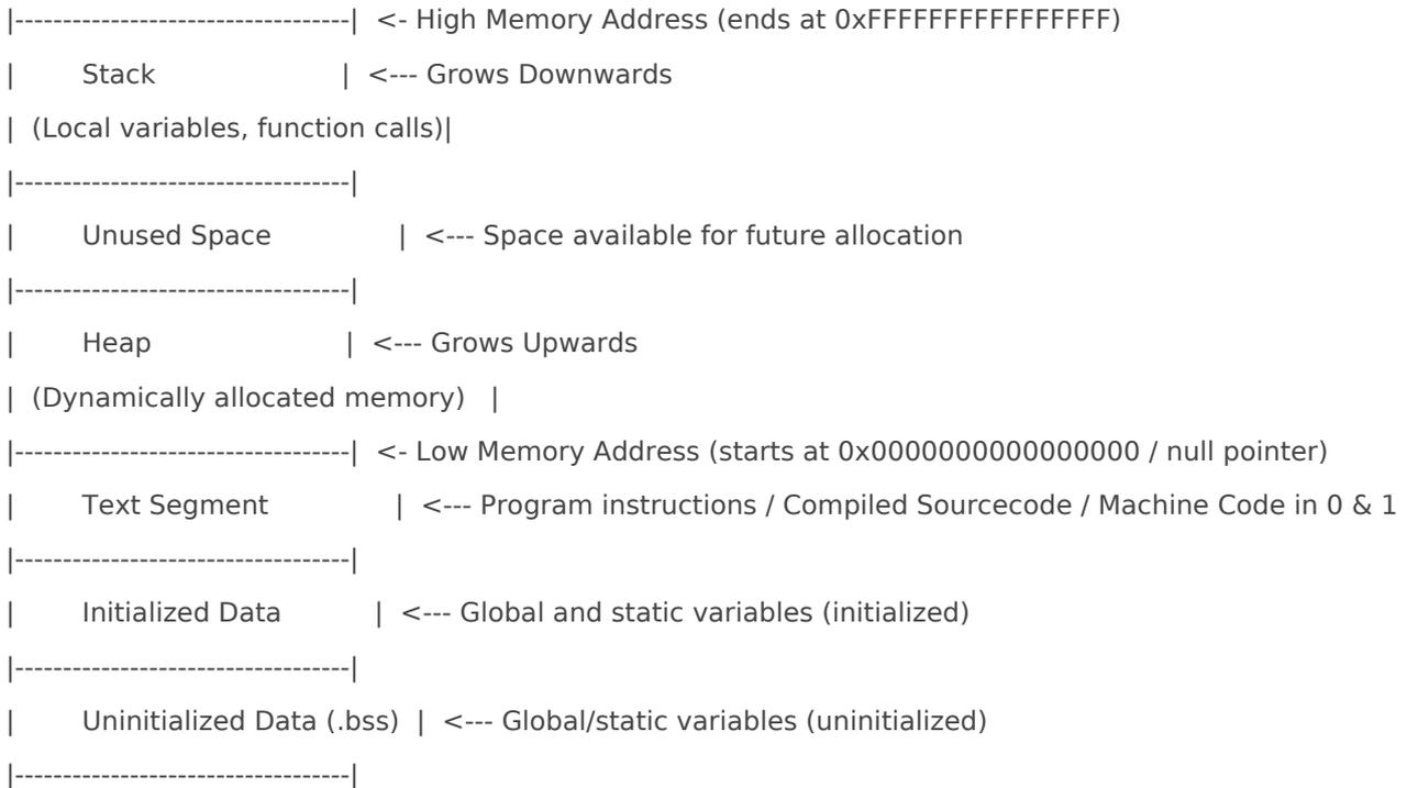
**Directionality Matters:** The upward growth of the heap and downward growth of the stack is crucial for efficient memory utilization, error detection, performance, and cache optimization.
